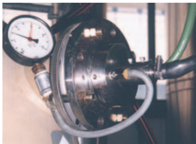
Fig. 5: High-pressure ejector for the transport of sorbents and dispersion in a reaction space
